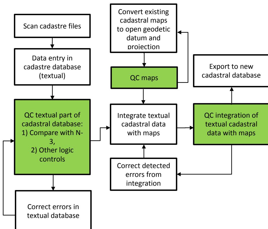
Figure 16 Digitization and integration of cadastral data workflow
