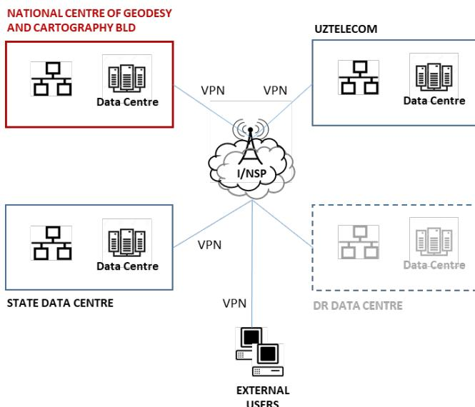
**Figure 12 Schematic Diagram of GKZGDK's WAN Architecture**
